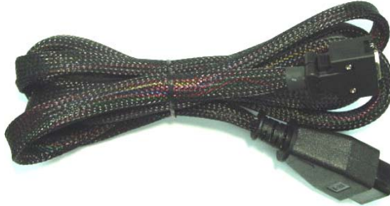
Figure 1.9 DLC Main Cable (16P)
